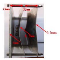
Fig. 27. Experimental result of flyer impact multi-layer structure
