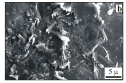
Fig. 13. The microstructure of the fiber tip surface after laser action. **a** - SEM image of a fragment of the fiber end surface; **b** - magnified SEM image of a fragment of the end surface with the crystal-like structures on the surface (Yusupov et al., 2011a).
